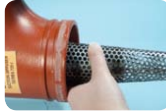
Remove basket, clean, then reinstall
